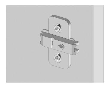
EURO version hinge guides (with an Euro screw in the set) must by screwed through the drilled holes (with a diameter of 5mm on the surface of the cabinet side).
