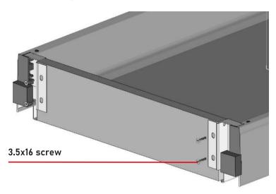
Screw the back of the drawer with the use of 3.5x16 screws (4/6 pieces depending on the height of the drawer back).
