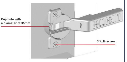
Place the hinge in the 35 mm cup hole prepared on the door surface. Screw the hinge to the doors with the use of two 3.5x16 mm screws.
