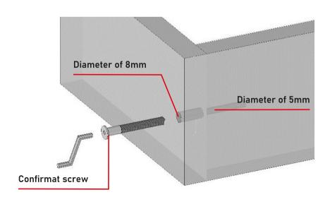
Put together two elements being fixed. Insert the  $6.4 \times 50$  confirmat to a hole with a diameter of 8mm (pas-through hole on the surface of the element) using a 4 mm hex key, screw the confirmat in the 5mm hole on the edge of the second element.
