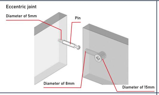
Insert the eccentric joint (cam lock) in a hole with a diameter of 15 mm (the arrow is directed towards the edge with the 8mm hole.
