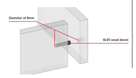
Put together two elements being fixed. Drive the dowel in the 8mm hole (hole on the edge of the element). Insert the element with the dowel to the 8mm hole on the surface of the other element.
