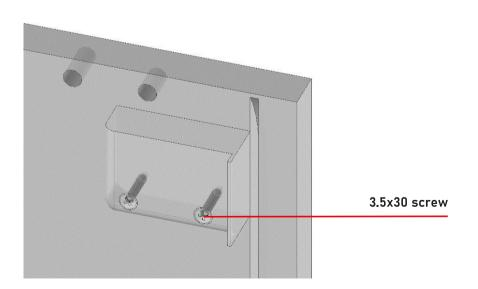
Screw the kitchen furniture mounting plate to the sides of the cabinet with the use of two 3.5x30 screws (there are two drilled holes next to the milled duct for the back wall).
