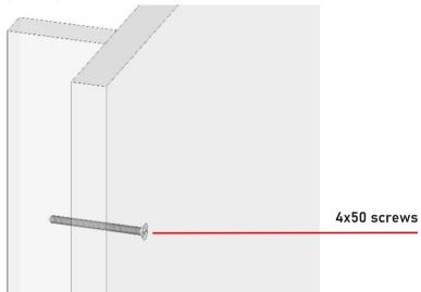
Screw the filler strip to the cabinet with the use of three 4x50 screws.
