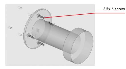
Kitchen furniture leg  $\,$  - screwed to the cabinet bottom panels with the use of four 3.5x16 screws.
